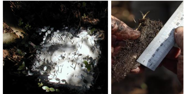
Figure 2. A Badu Mangroves feldspar marker horizon at installation (a) and soil core retrieved from the plot 17 years later, showing 7cm of organic and sediment accretion.
